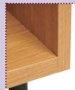
8mm solid back, 18mm thick vertical MFC panels, 1mm ABS on leading edges
